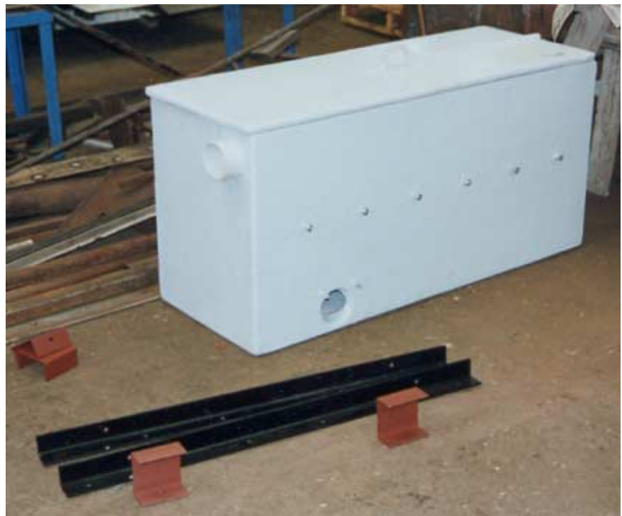
Completed tank with mounting brackets. The angle iron bolts to the tank. The short channel sections bolt between the angle iron and the carriage underframe.
