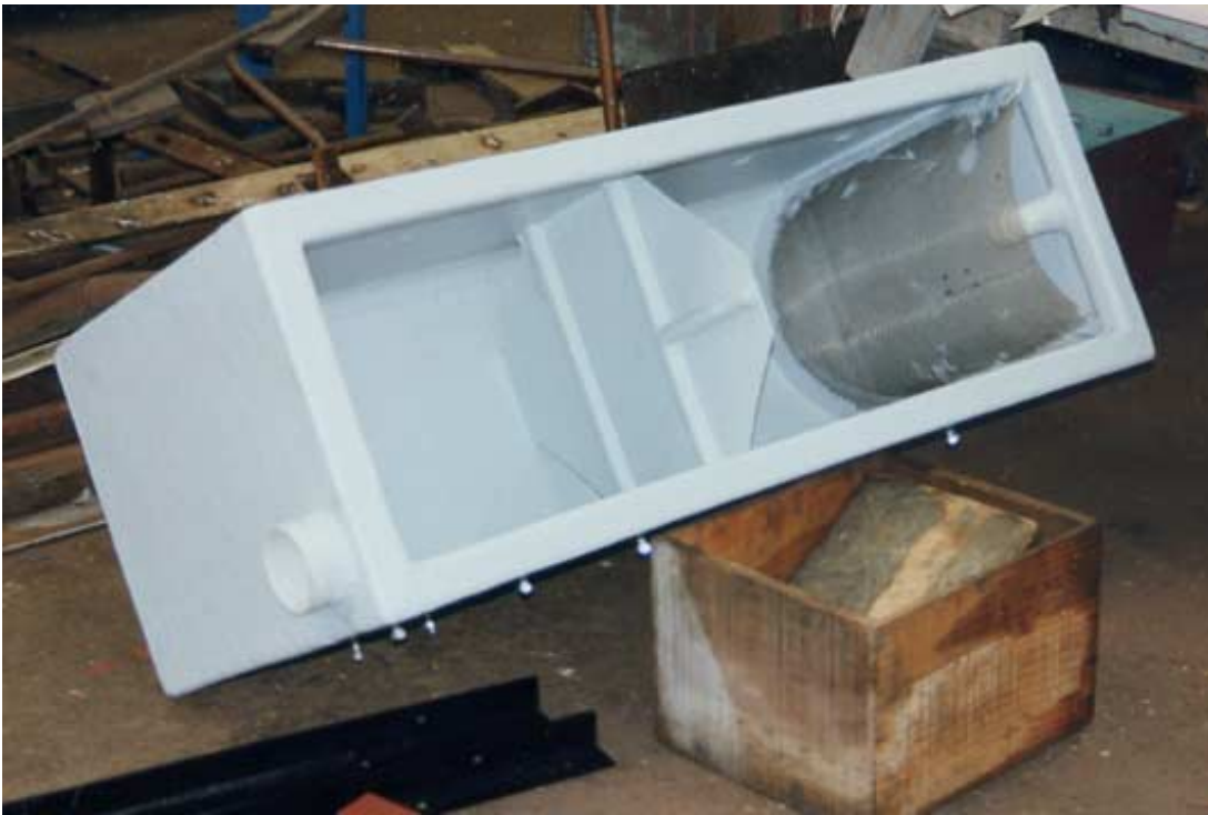
Interior of tank showing baffle and screen.
